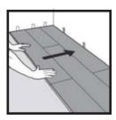
**9.** Once you have installed 2-3 rows, make adjustments to the distance between the floorboards and the front wall by placing 1/4" spacers. Keep the spacers in place throughout the installation process and remove them only after the installation is complete.
