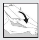
**7.** Position the short end of the floorboard at an angle against the previously installed floorboard in the second row and proceed to fold it down entirely as the second plank of the second row.
