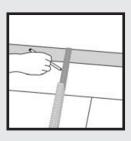
**10.** In case the wall is uneven, the floorboards need to be adjusted to fit its contours. To achieve this, mark the floorboards with the contour of the wall, ensuring to leave a 1/4" space between the floorboards and the wall. This process should also be followed for the first row if required.
