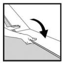
**2.** For the second plank in the first row, angle the short end towards the first plank and press them together before laying it down. Repeat this process to complete the first row.
