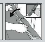
**11.** Using a chisel, remove the locking element from the adjusted strip, and apply the appropriate glue to it.
