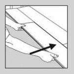
**8.** Slide the plank forward by applying pressure, so that it aligns with the first plank in the row.
