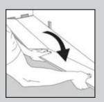
**7.** Position the short end of the floorboard at an angle against the previously installed floorboard in the second row and proceed to fold it down entirely as the second plank of the second row.
