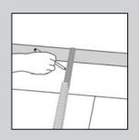
**10.** In case the wall is uneven, the floorboards need to be adjusted to fit its contours. To achieve this, mark the floorboards with the contour of the wall, ensuring to leave a 1/4" space between the floorboards and the wall. This process should also be followed for the first row if required.
