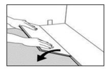
**6.** To install a floorboard, angle it against the previous row's floorboard, press forward, and fold it down simultaneously. Leave the panel in a slightly upward angled position where the panels start to lock.
