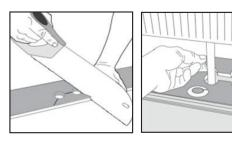
**12.** To create holes for the pipes, mark the center of the hole and drill it with a diameter approximately 16mm larger than the pipe's diameter, leaving a 1/4" gap around the pipe. Cut the plank as indicated using either a saw or a sharp utility knife and proceed to install it. If required, apply glue to the cut piece and replace it in its original position.
