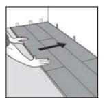
**9.** Once you have installed 2-3 rows, make adjustments to the distance between the floorboards and the front wall by placing 1/4" spacers. Keep the spacers in place throughout the installation process and remove them only after the installation is complete.
