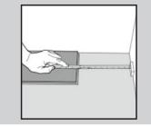
**3.** At the end of the first row, place a 1/4" spacer against the wall and measure the remaining space to determine the length of the last plank needed. Cut the last plank to the correct length, ensuring that it is at least twice the width of the plank for optimal installation.
